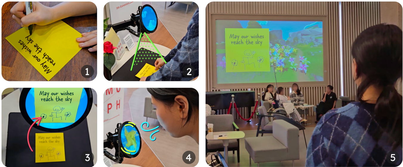
Figure 1: Overview of the interactive system. (1) A user writes a wish on colored paper. (2) The paper is placed under the circular display. (3) The system detects the paper, displaying it on the screen and digitally folding it into a pinwheel shape. (4) The user blows toward the circular display to rotate the virtual pinwheel. (5) After the interaction, the pinwheel flies to the shared virtual field on the main display and later unfolds to reveal the message.
