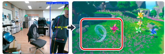
Figure 3: Position-synchronized visual feedback. A visitor’s physical position is mapped to a corresponding wind effect in the shared virtual field.
